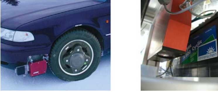
Fig. 14 Left: Laser triangulation sensor for friction prognosis [16], right: Laser triangulation sensor used in the measuring platform.
